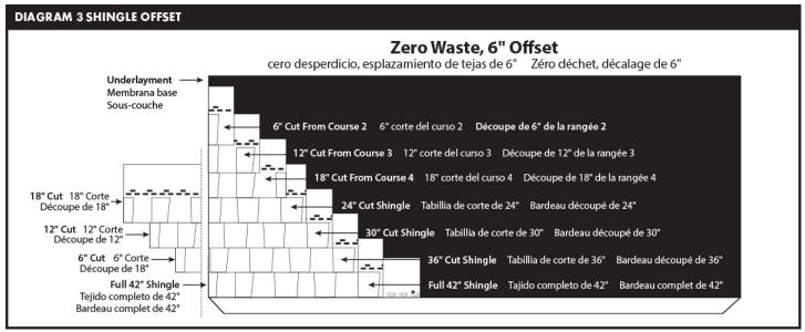
**Second Course:** Cut 6" off the left end of a shingle and apply the remaining larger piece over the first course shingle, flush with the left edge and exposing the first course 6". Proceed with full shingle across roof maintaining 6" exposure. Save the 6" piece for starting course 7. See Diagram #3.
