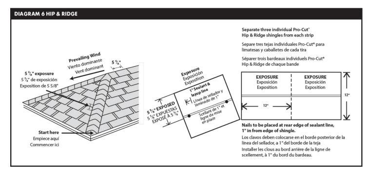
Separate the Pro-Cut<sup>®</sup> Hip & Ridge shingle into three equal pieces along the perforated lines provided. Bend each piece lengthwise to provide equal exposure on both sides of the ridge. Allow 5-5/8" of exposure and nail 6" from exposed butt edge with 2 nails 1" from each side. The direction of the exposed end should be away from the prevailing wind. One bundle of shingles will provide approximately 31 lineal feet of ridge coverage when applied in accordance with these instructions.
