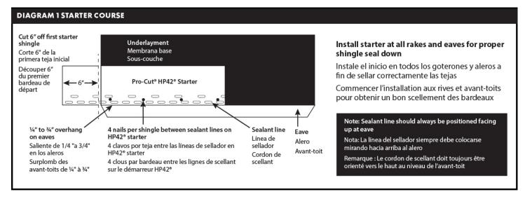
**First Course:** Begin first full shingle at lower left rake of roof or right of vertical chalk line and continue course across roof with full shingles laid flush with starter course and fastened with 4 nails, placed as specified. Note: an optional band of asphalt plastic cement meeting ASTM D-4586 may be applied to the rake of the roof with each shingle course to enhance wind resistance and to resist wind driven rain infiltration. See Diagram #3.
