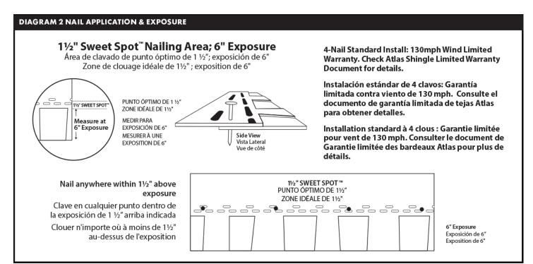
RE-ROOFING APPLICATION (second shingle layer): Requires the same nail placement as New Roofing.
