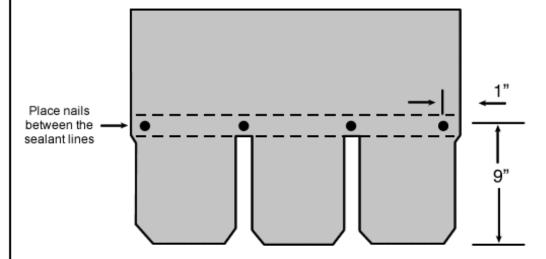
NAIL PLACEMENT IS IMPORTANT FOR WIND RESISTANCE. INCORRECTLY PLACED NAILS WILL VOID WIND COVERAGE OF WARRANTY.
