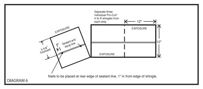
When installing ridge vents follow vent manufacturer's instructions. The direction of the exposed end of the ridge shingle should be away from the prevailing wind. One bundle of shingles will provide approximately 31 lineal feet of ridge coverage when applied in accordance with these instructions.
